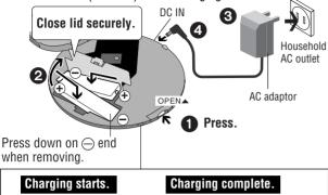
The "CHG" lamp lights. The "CHG" lamp goes out. During charging, " 📋 " scrolls on the remote control.
