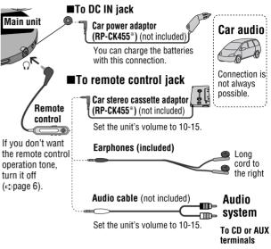
\*The RP-CK455 set contains the car power adaptor and car stereo cassette adaptor. Be sure to use these together with the car audio connection.
